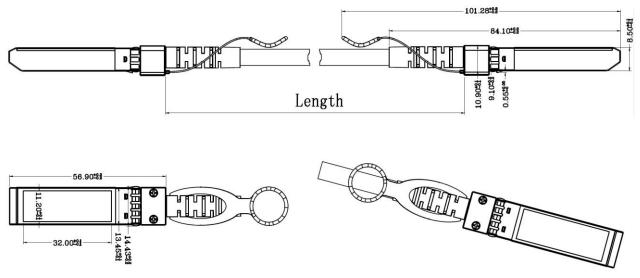
**Diagram of Mechanical Dimensions**
