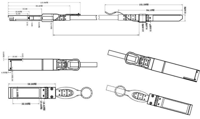
Diagram of Mechanical Dimensions
